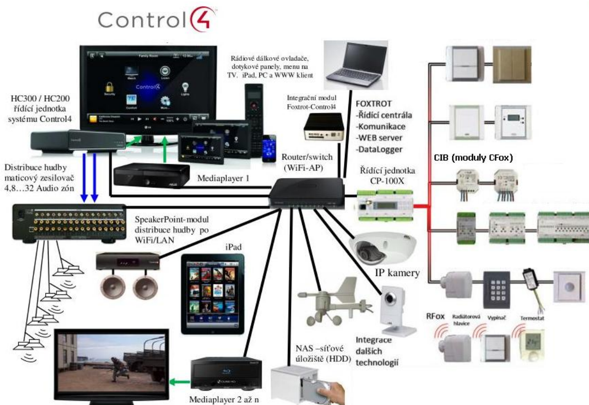
Fig. 9.4.1.1 An example illustrating the interconnection of the Control4 and Foxtrot systems
