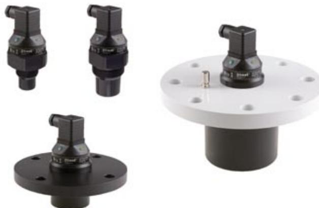
**Ultrasonic level meters ULM®** is self contained device that includes electroacoustics transducer and electronic module. The level meter ULM transmits series of ultrasonic pulses which propagates towards the liquid surface. Reflected acoustic wave is received back in the ULM transducer and processed in electronic module. The distance calculations are based on time of flight of the acoustic wave to the level and back.
