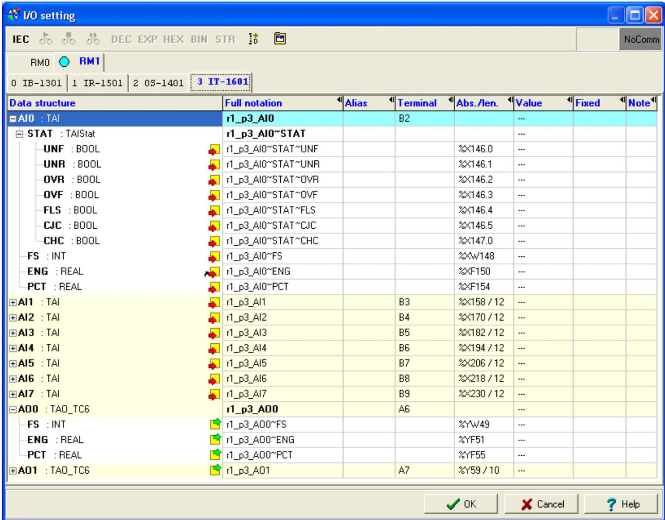
Fig.3.4.4 IT-1601 module data structure
