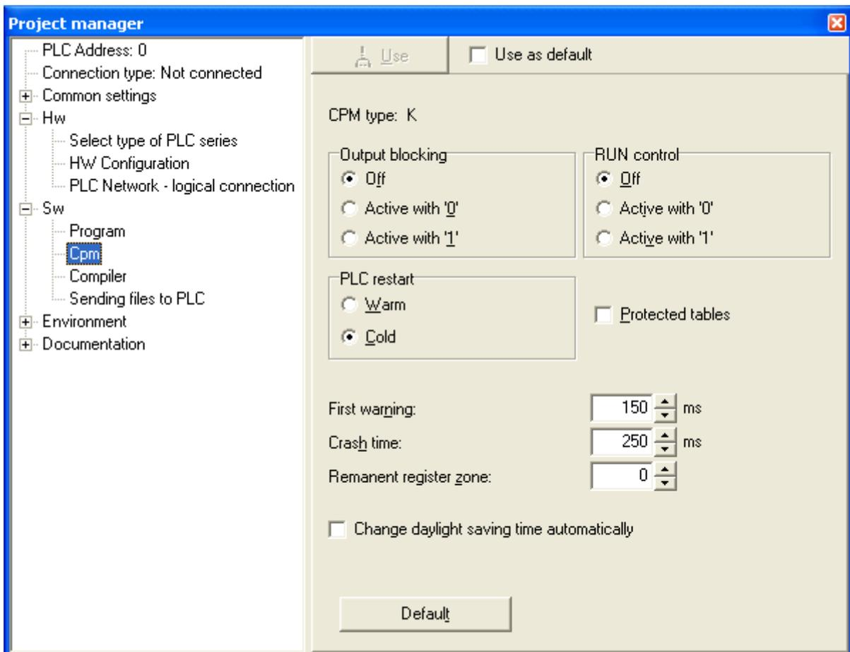
Fig.5.1 Configuration constants setting
