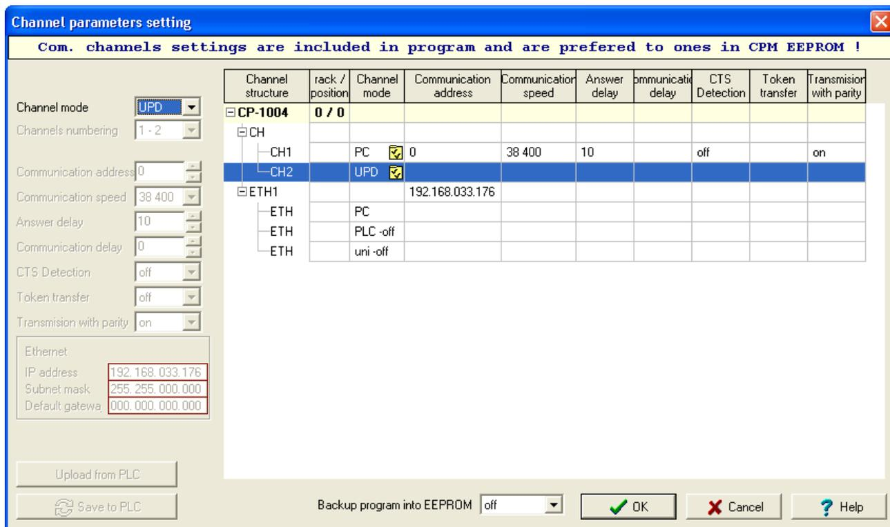
Fig. 2.5 UPD mode selection in the channel CH2
