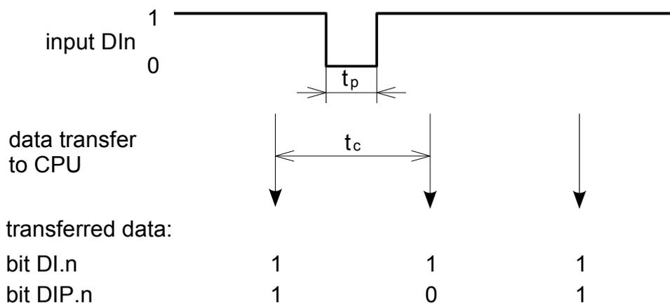
**Fig.3.1.8** Detection of short impulses into log.0 function
