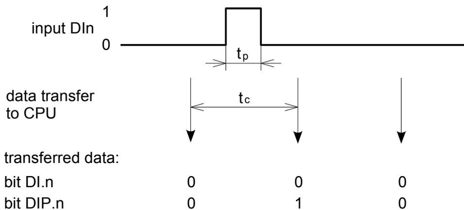
Fig.2.20 Detection of short impulses into log.1 function
