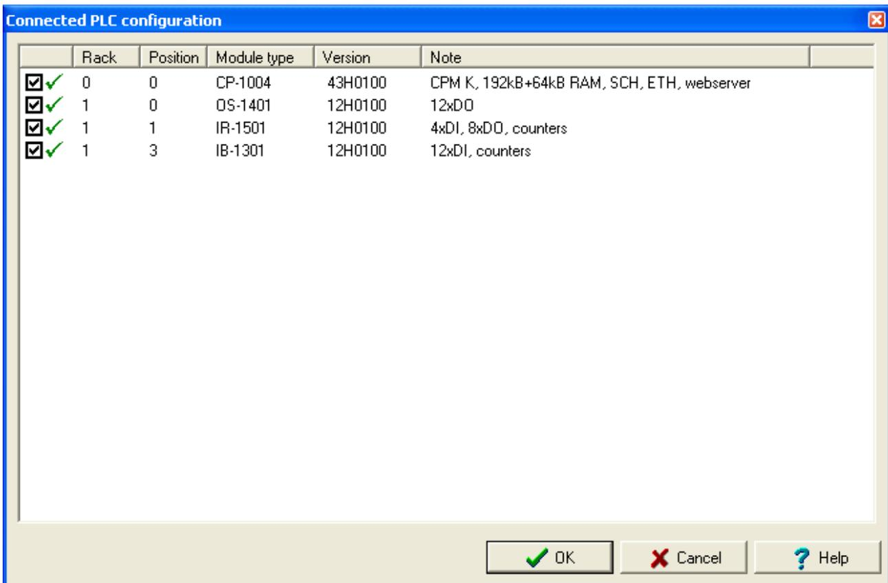
*Fig.5.5 Download of configuration from PLC*
