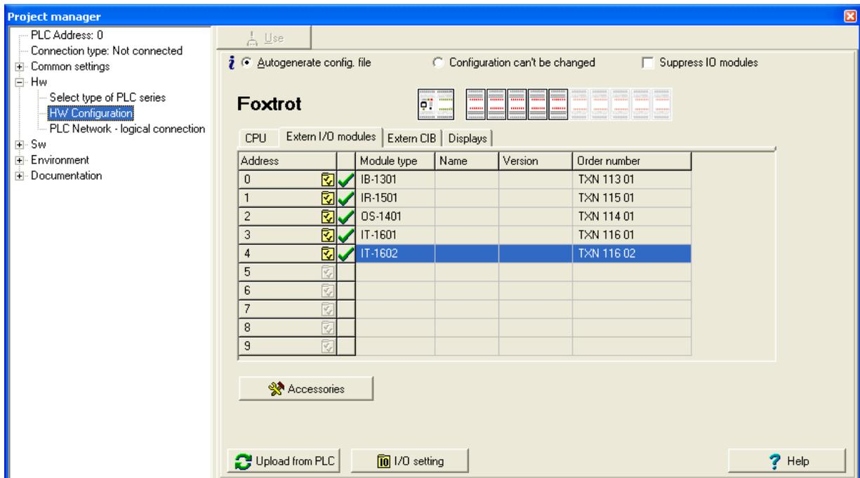
Fig.5.4 PLC FOXTROT configuration settings- peripheral module
