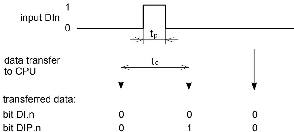
Fig.3.3.10 Detection of short impulses into log.1 function
