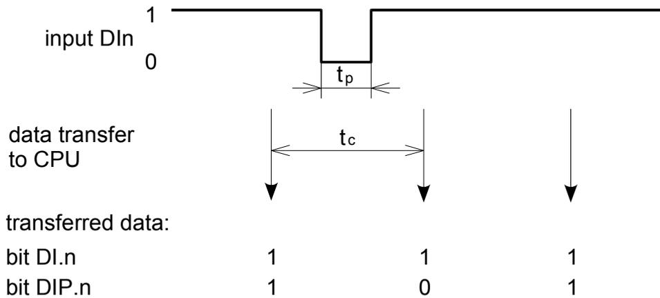
Fig.2.19 Detection of short impulses into log.0 function
