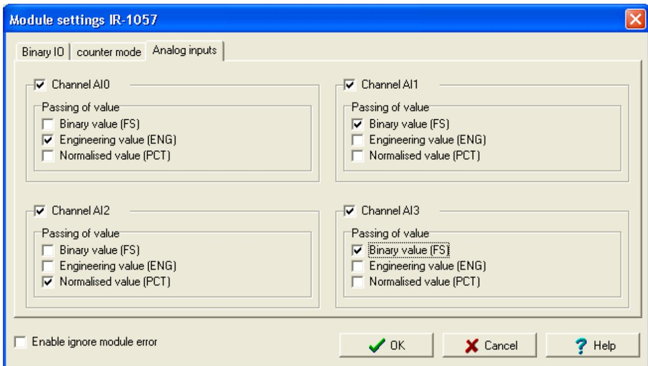
Fig.2.21 Configuration of analog inputs
