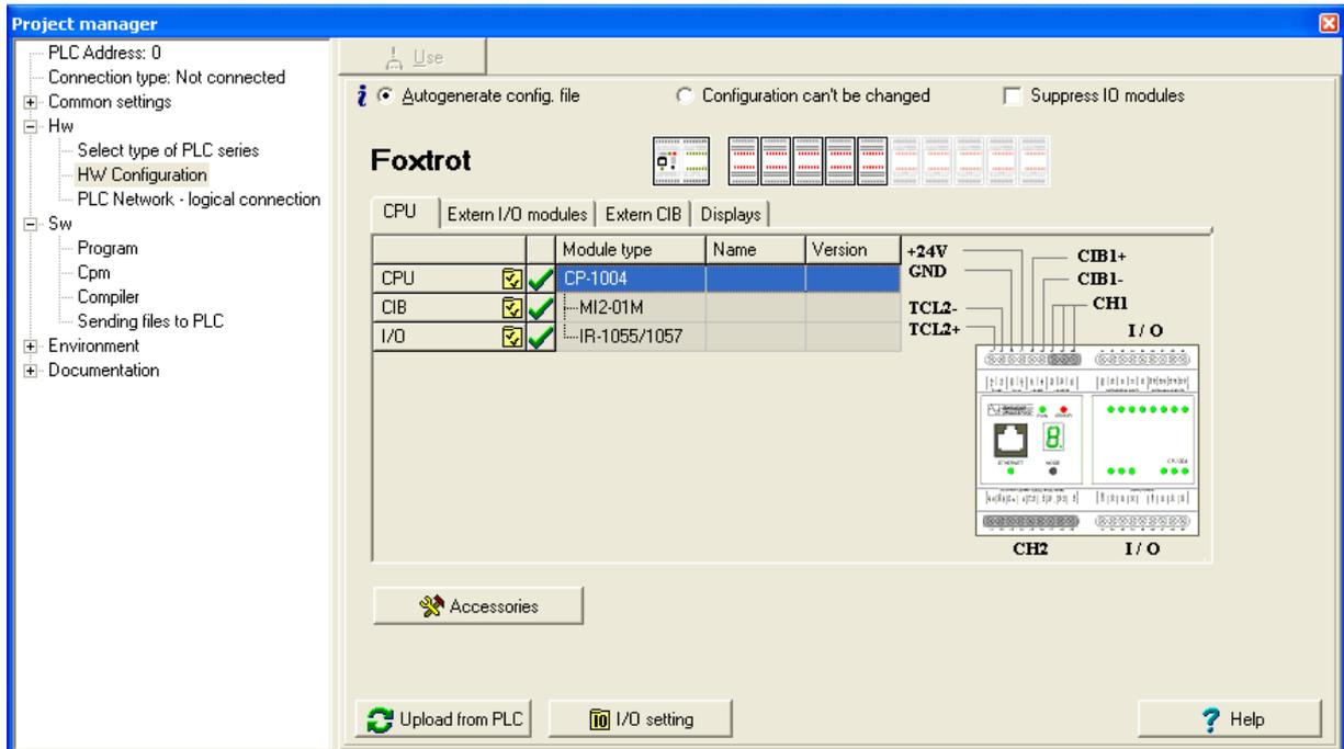
Fig.5.3 PLC FOXTROT configuration settings- basic module
