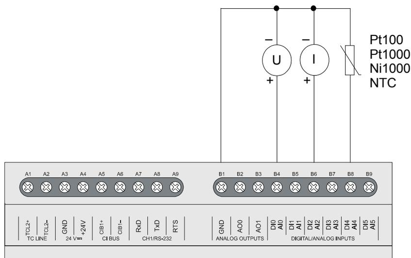
Fig.2.28 Typical example of signals connection to analog inputs of basic modules CP-1005, CP-1015 (individual signal types are connectable to any analog
