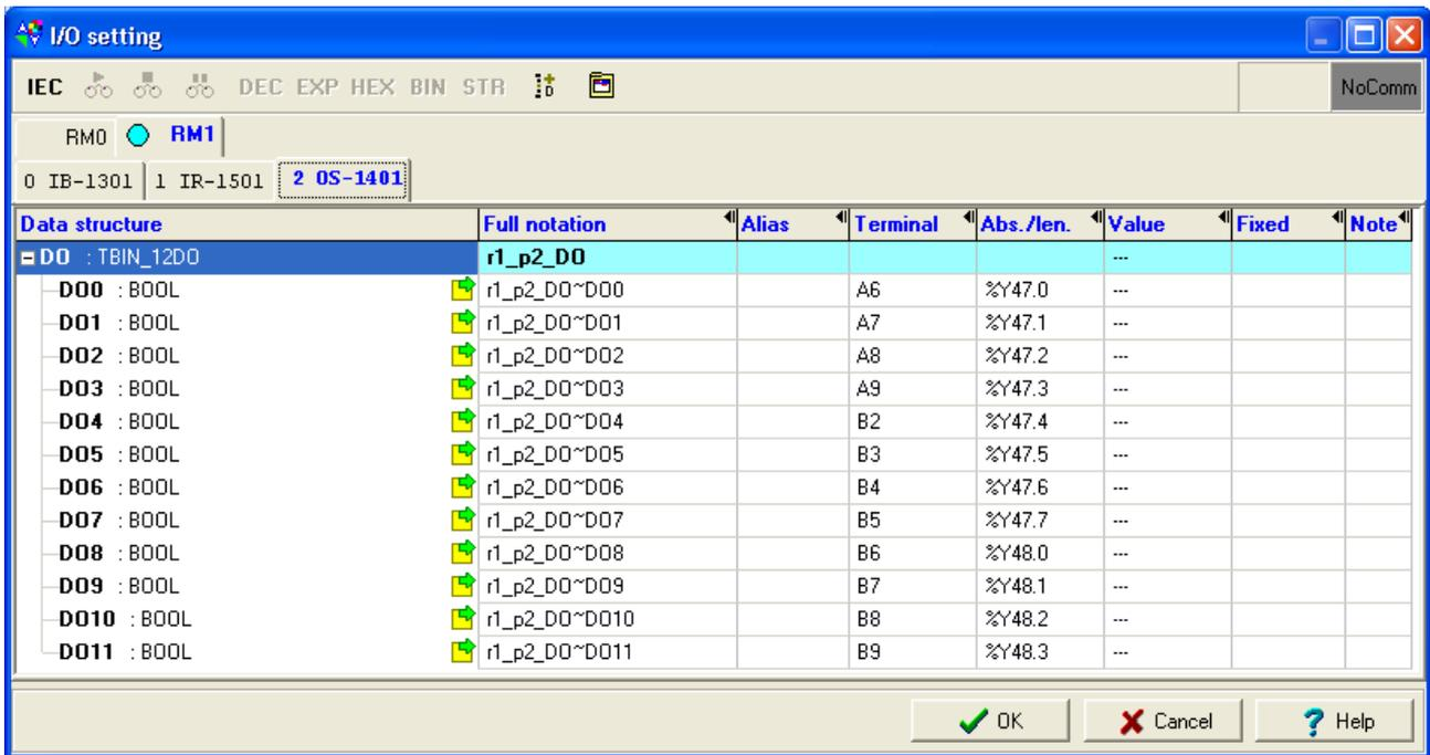
Fig.3.2.3 OS-1401 module data structure
