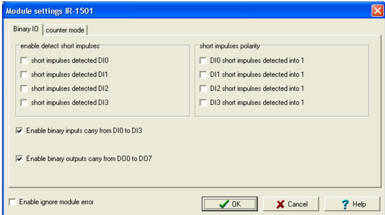
Fig.3.3.8 Configuration of binary inputs and outputs
