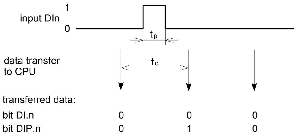
**Fig.3.1.9** Detection of short impulses into log.1 function
