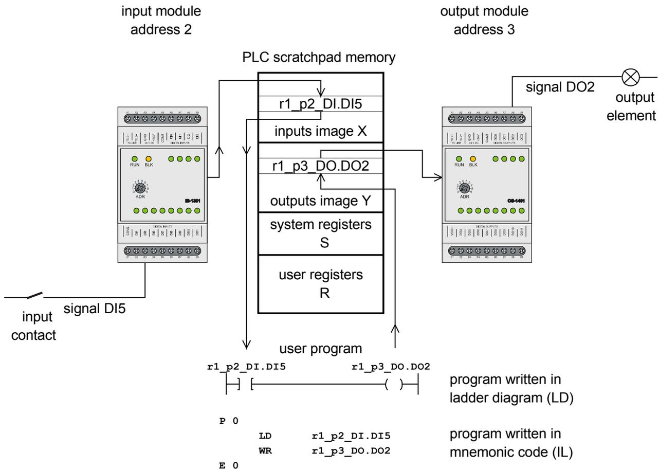
Fig.1.2 Signal processing scheme of the PLC
