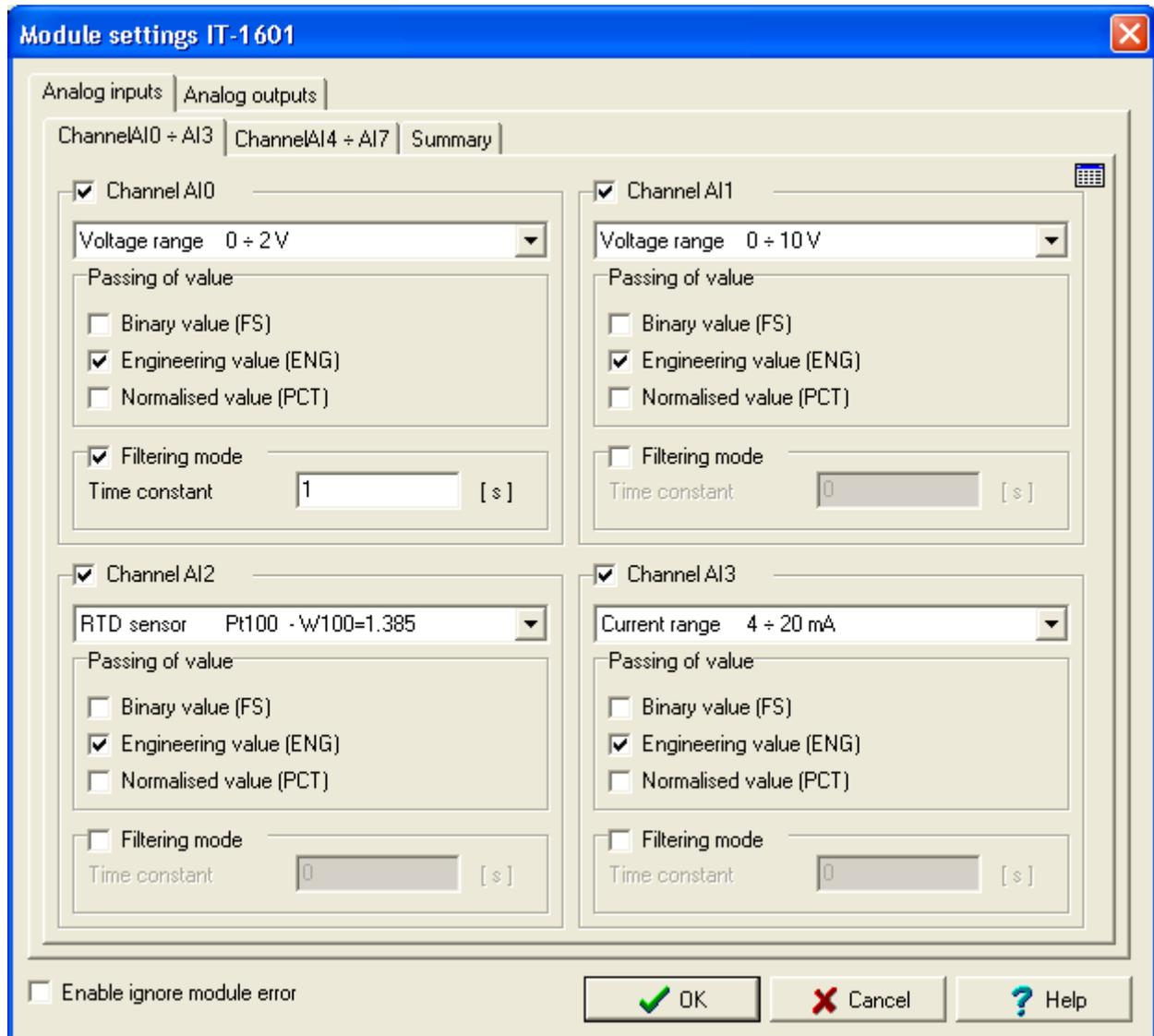
Fig.3.4.6 Analog inputs configuration
