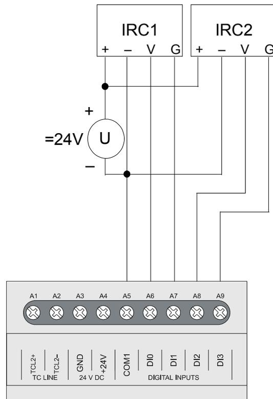
Fig.3.3.4 Example of two IRC position sensors connection
