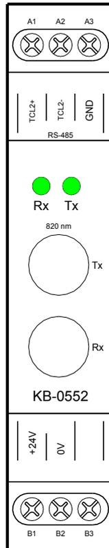
Fig.4.1 Optical interconnection module KB-0552
