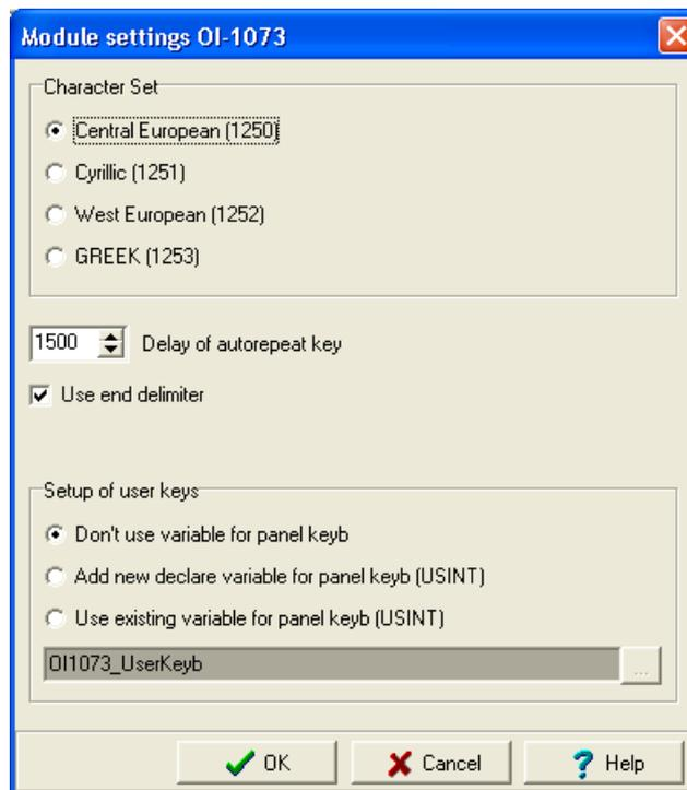
Fig.2.44 The OI-1073 display configuration
