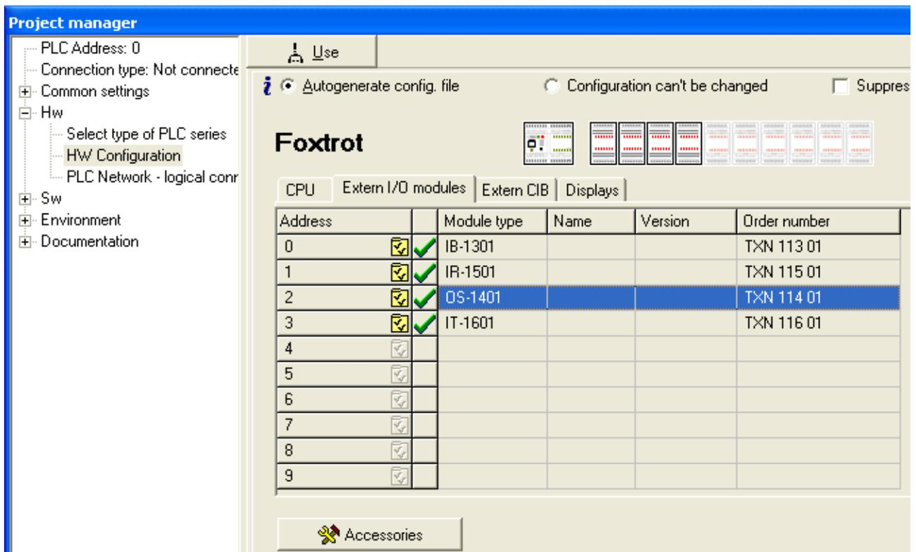
Fig.3.2.4 Configuration of peripheral modules
