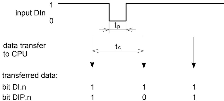
Fig.3.3.9 Detection of short impulses into log.0 function
