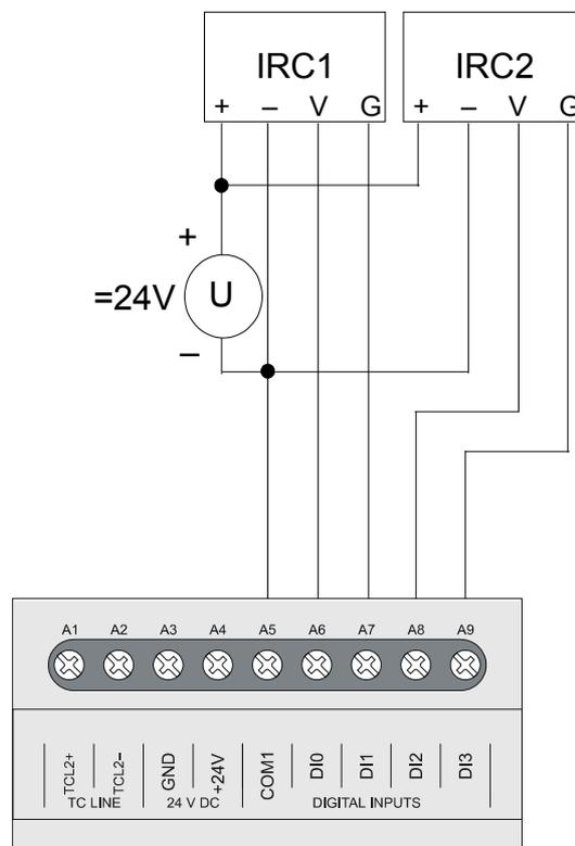
*Fig.3.1.3 Example of two IRC incremental encoders connection*
