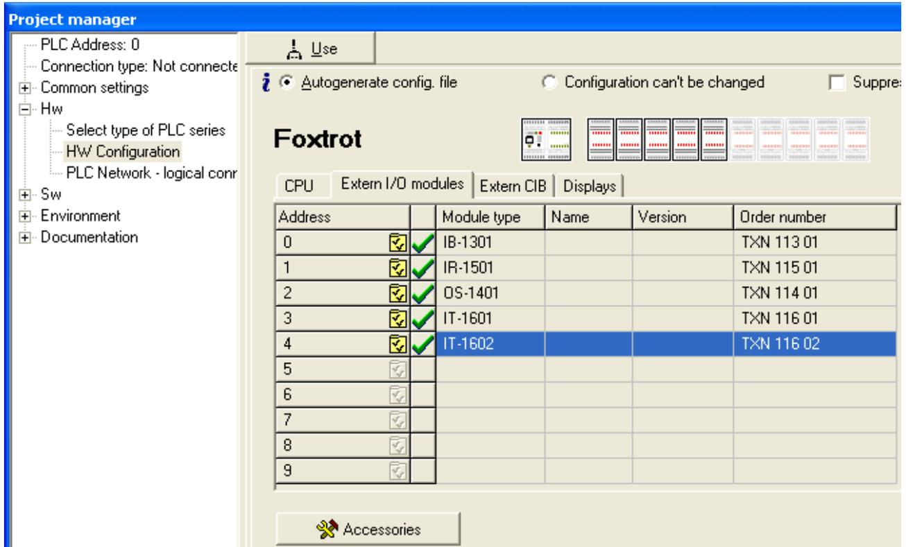
Fig.3.4.18 Peripheral modules configuration
