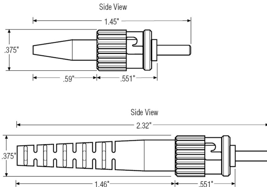
Fig.4.2 Mechanical dimensions of the ST optical connector
