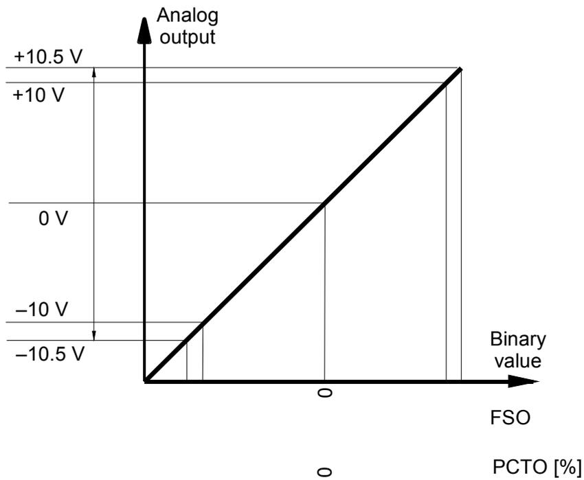
Fig.3.4.23 Analog outputs range of the IT-1602 module
