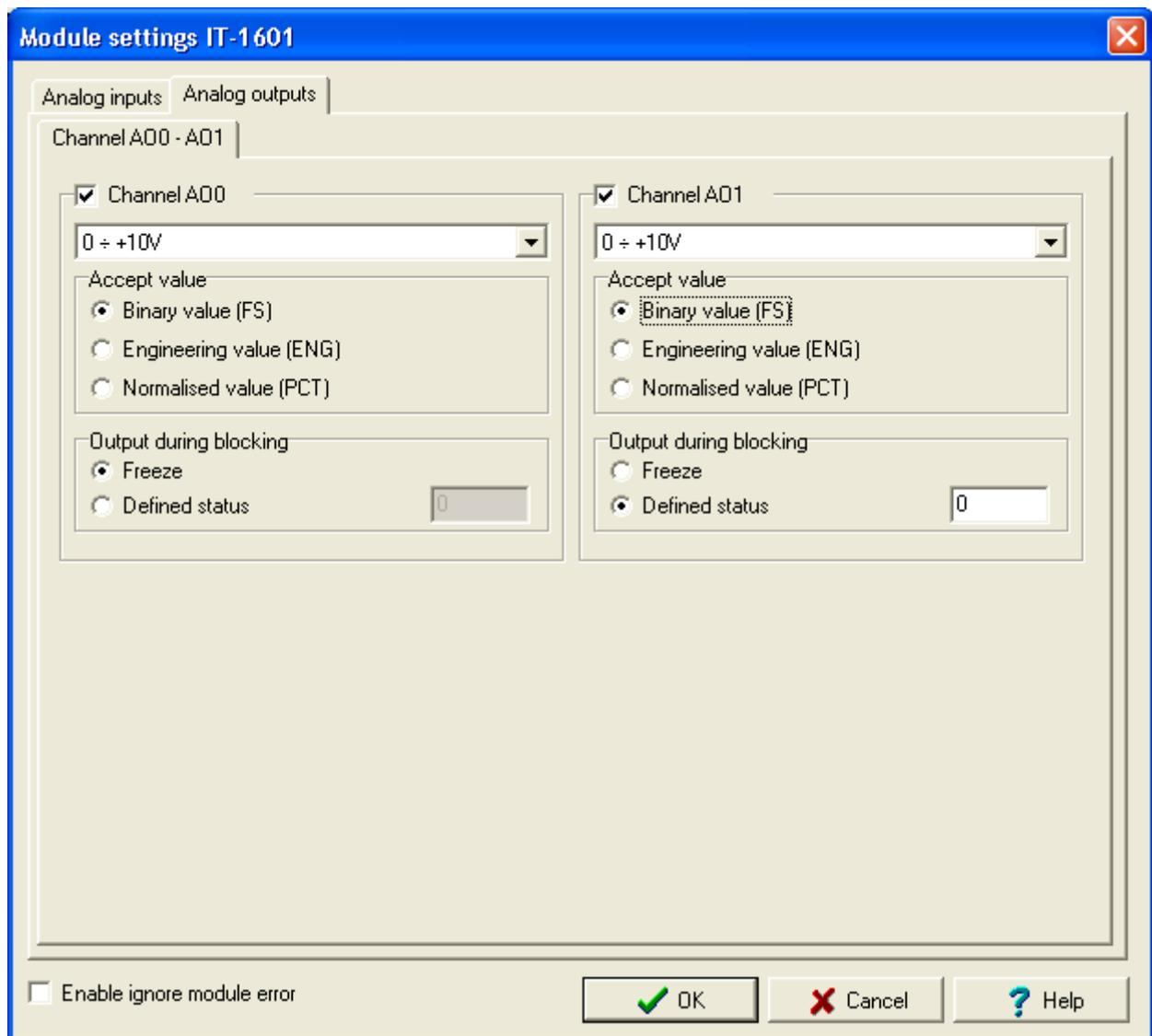
Fig.3.4.12 Analog outputs configuration
