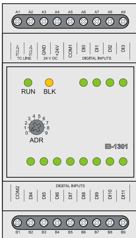
Fig.3.1.1 Peripheral module IB-1301
