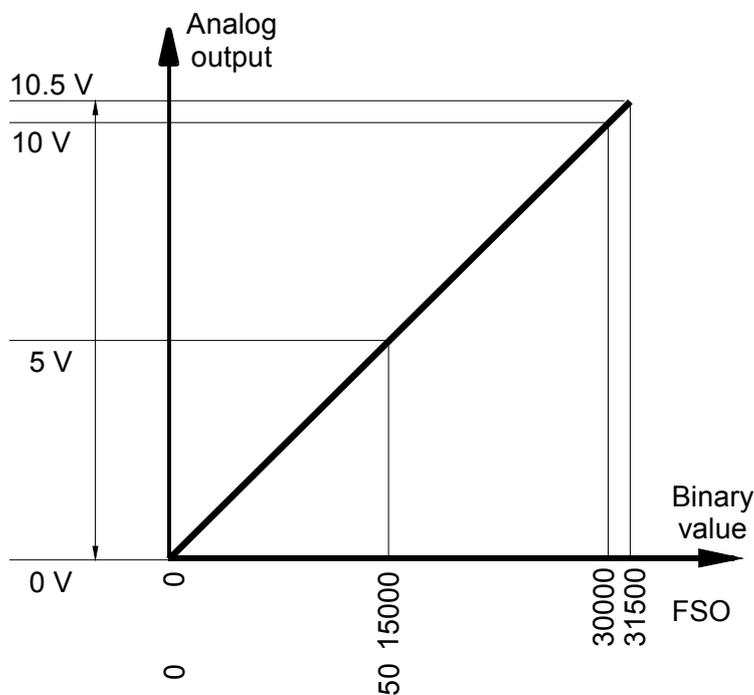
Fig.3.4.13 Analog outputs range of the IT-1601 module
