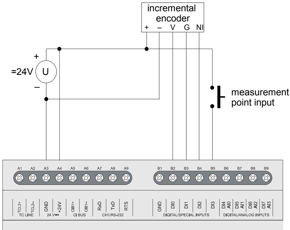
Fig.2.15 Example of the IRC incremental encoder complete connection
