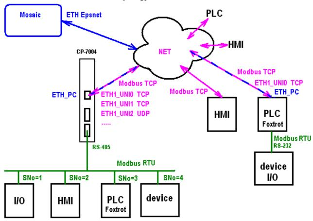
Serial line communication can work as Master-Slave on more channels simultaneously. In Ethernet network it is possible to combine different communications among devices. A master can direct its communications to eight slave devices with various IP addresses at a time. There can run any other communication for example with development environment Mosaic or another PLC at the same time.
