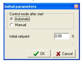
In the dialog you can set up a status in which the regulator will be after start of the system. There can be chosen automatic or manual mode. Depending on this option and mode of the regulator there can be set an initial desired value, initial action intervention or an initial desired proportion.
