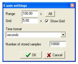
The axis range in seconds can be set in the dialog. The pushbutton "All" sets the range so that all the measured data are displayed.
