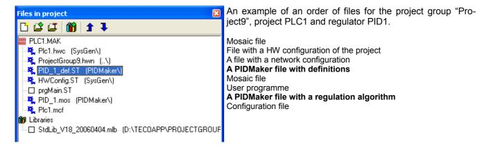
An unique group of variables is established for each regulator; their names are in an unified format according to the rule "<regulator name>\_<variable name>", e.g. "PID1\_Input1". In acse there is chosen "Establish a structure above regulator data", it is possible to access the variables through the structure named "<regulator name> struct".
