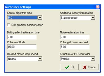
Type of regulation algorithm – this pop-up window with options allows choosing a type of the regulation algorithm PI or PID, for which the auto-tuner will estimate parameters.
