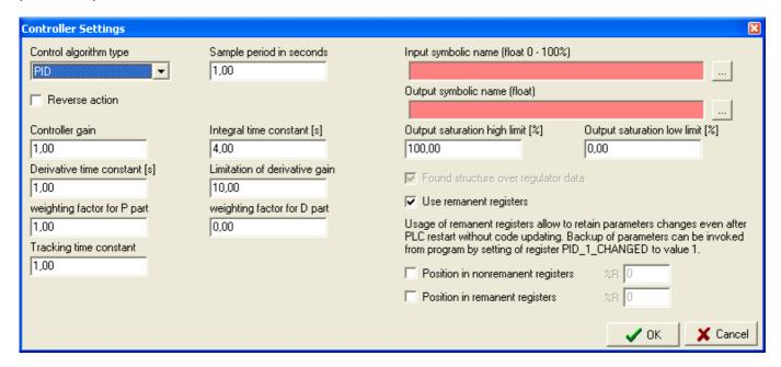
Type of regulation algorithm – the pop-up window allows choosing a regulation algorithm of the type P, I, D, PI, PD, ID, PID. The abbreviations define which of the PID algorithm components will be active. Automatic setting of the parameters is accessible only for the PI and PID algorithms.
