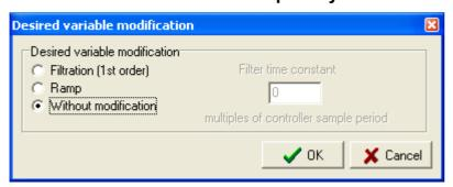
Without modification = the entered desired value is used directly for calculation of the regulating deviation.
