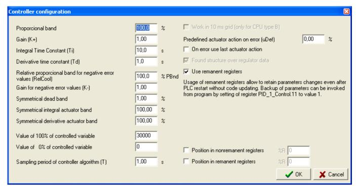
Proportionality band (PBnd) (0.1 to 3000%) – this gives indirectly amplification of the regulator. This item is bound with entered amplification by the following relation:
