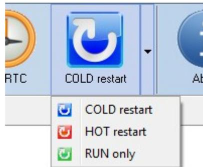
Except both types of restart a user can also select transition to RUN status, when PLC system programme is launched without restart, in other words without any memory initialization. *RUN only* in the menu corresponds to this function. After choosing one of the offered options and PLC system selection in a list of available devices, device restart or *RUN only* transition can be done by pressing abutton in a toolbar. The process is indicated by *Restarting* dialogue.
