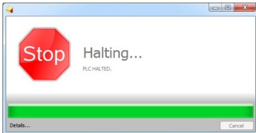
At this moment everything is prepared for a new project loading to a selected PLC device. First of all files from *SendRoot* folder are transferred to a system memory card. The operation can take several minutes if there are a lot of transferred data. It is followed by loading of databox and remanent registers contents, if they are required by the project, finally the machine code including the configuration charts is loaded. Partial steps process can be seen in *Loading* dialogue.
